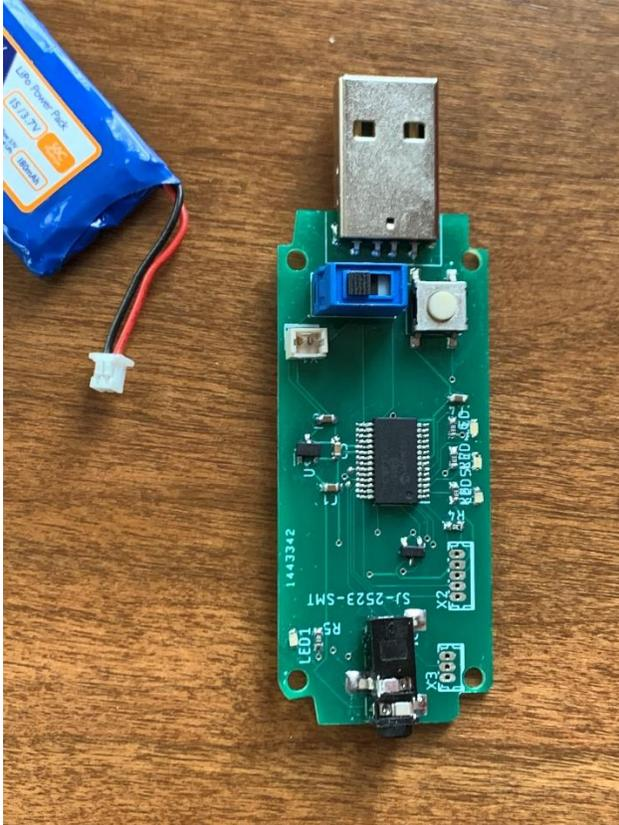
When you look at the connector you will see the black negative wire. The connector is polarized so that goes in with negative wire on the outside edge of the board. It is a locking connector that will snap in.
