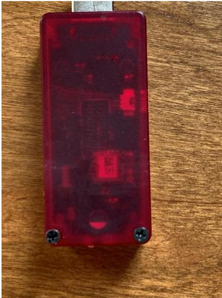
The next step is to take the circuit board out of the top casing. It is held on by two screws at the USB end
