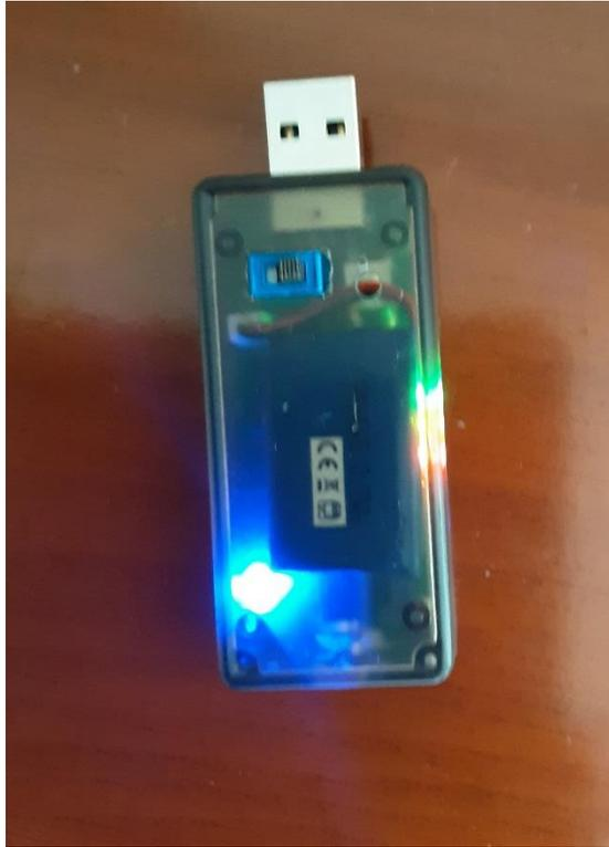
Now your turn on the Dongle and timer. You can power the timer from either a USB power source or from an internal LiPo battery.
